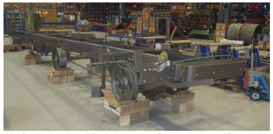
View from the downside end: This is the same **base frame version as modified in 1912**, where the water tanks were removed (by Bell, Kriens) and the lower two axis mounted initially in a bogie were replaced by a stiff arrangement with the **middle axis having no wheel flanges**. All steel parts were sand blasted and have a new paint. Photo HW, 2020-02-25
